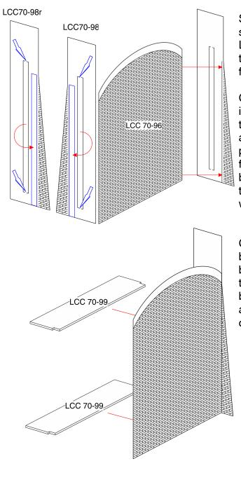
Start by cutting out the long strip from LCC 70-98l and LCC 70-98r. Proceed to glue the strip in marked location flush with the engraved line.
