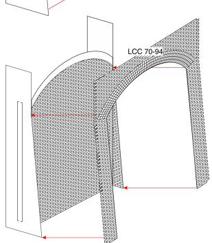
Finally finish the base assembly by gluing the face panel to the back assembly. The material used to make this model is flexible and will bend easily to the shape of the back assembly. Do not use excessive force and let the front panel follow the curvature of LCC 70-98I and LCC 70-98r.
